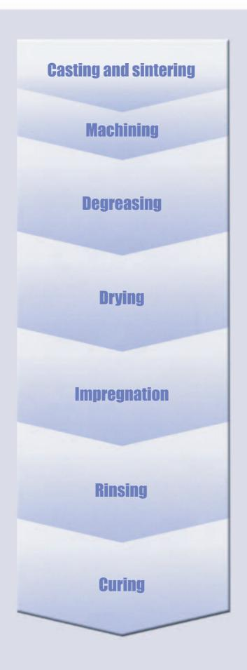
Impregnation is usually performed after machining and heat treatment. Since cutting oil and other cutting enhancers adhere to the surface of the workpiece and may even penetrate defect interiors, these materials should be removed by dry-heating or rinsing.
